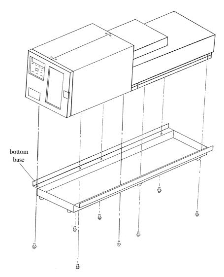
Figure 1-10. Attach to Bottom Base
